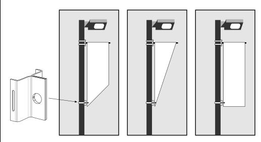
The mount is perfect for use with pennant-style banners where the KBW BannerFlex banner bracket is installed at the top hem and the new Tie-down Mount is installed at the lower corner. Additional Tie-Down Mounts may be installed on longer banners along the pole side if desired.
